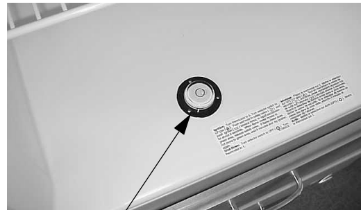
Place bubble level in bottom of refrigerator
