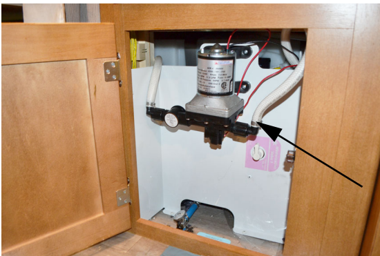
Water Pump (Located behind access door in bottom of pantry) *Models 22M -Typical View
