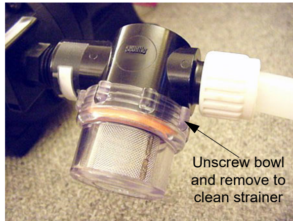
Water Pump Strainer -Typical View
